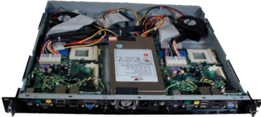
The ITOX Twin Dragon 1U rackmount platform contains two advanced motherboards, each with its own 3.5" drive bay and Ethernet LAN controller. Two Twin Dragons can fit back-to-back—enabling 4 servers to fit in a single 1U space and 168 servers in a 42U rack. The Twin Dragon is available as a barebones platform (case, power supply, and motherboards) or a full system including your choice of CPU, memory, hard drive and operating system.
