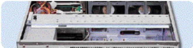
PRC-4184 adopts the newly designed card retainer to hold both the PCI and ISA type add-on-cards more tightly.
