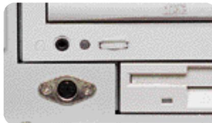
PRC-4184 is equipped with one PS/2 type keyboard connector inside the front panel to have a better security control.
