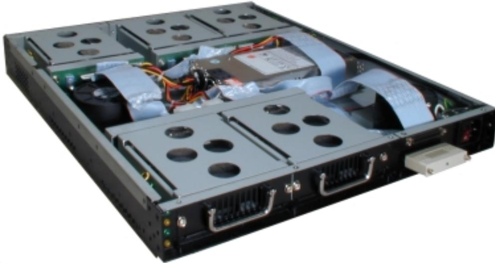
The ITOX Dragon RAID 1U Storage Platform provides five externally accessible, hot-swap bays and metal drive carriers for SCSI drives. ITOX offers the Dragon RAID as a case only platform (case, drive carriers, power supply) or a full system (including drives). A complete RAID system requires a RAID controller card, which resides in a host PC and a data cable from the host system to the Dragon RAID.
