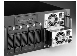
Front-access and hot-swap redundant 400 W ATX power supply for easy maintenance.
