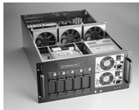
Hot-swappable cooling fan assembly installed on the middle of the chassis.
