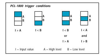
This control logic (all software programmable) lets you set up complex alarm and triggering conditions. For example, you can set the watchdog to trigger if the input is either above the high-level value or below the low-level value. You can also set the PCL-1800 for rising or falling edge triggering.
