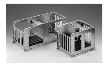
The IPC-6006 series are open-frame card cages with a 6-slot ISA or ISA/PCI backplane. They are especially suitable for OEMs who wish to customize the appearance of their PC-based systems. The IPC-6006 can hold 6 full-length cards, and the IPC-6006S can hold 6 half size cards. They have pre-punched mounting holes for a PS/2 power supply and one 3.5" HDD, allowing for easy system integration.
