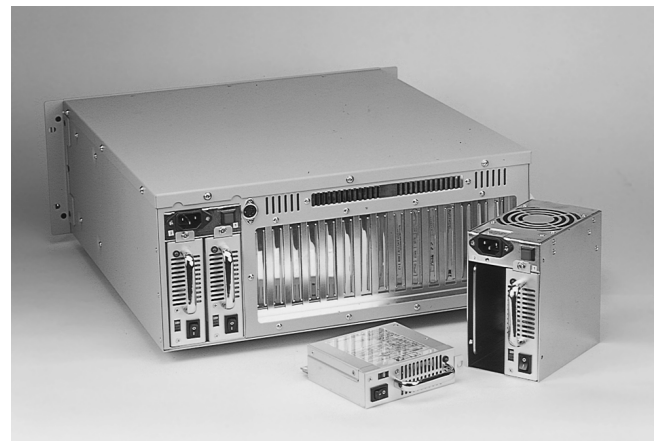
The IPC-615 is equipped with a 250 W hot swap redundant power supply. If one fails, the other will take the full load automatically.
