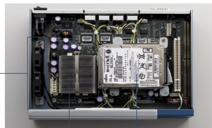
Intel Celeron CPU 2.5" IDE HDD space
